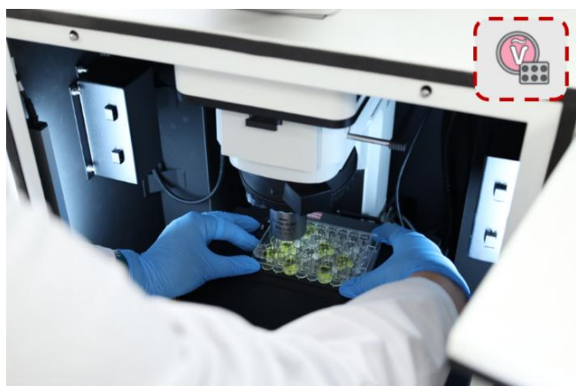
Figure 1. Multi-well plate analysis on RMS1000 Confocal Multimodal Microscope.
