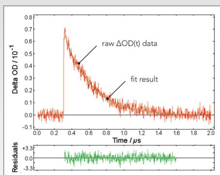
The sample being investigated is exposed to an intense laser pump pulse, which creates the transient species, and the probe source, which forms the background for the time dependent absorption measurement.
