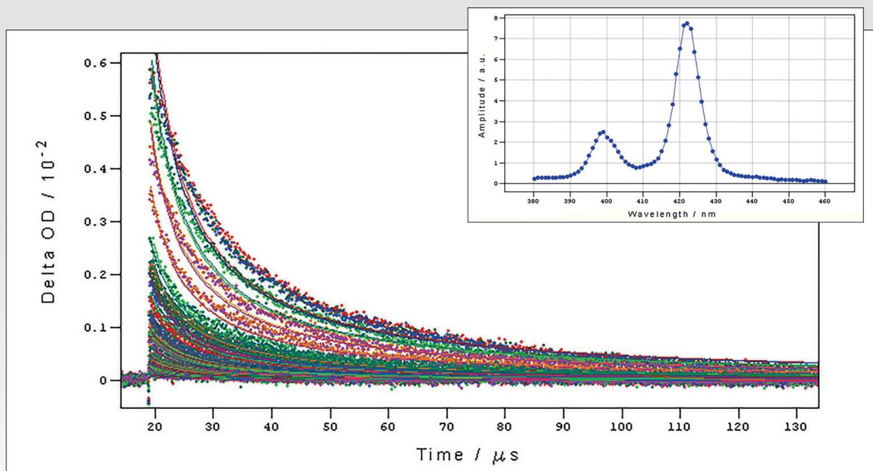
Raw data and fitted curves of the set of 80 time-resolved measurements of an anthracene example. Data were analysed with FLASH software (optional) using Global Analysis of a second order kinetic decay model, globally linking the rate constant. The result of the fit is a global second order rate constant of  $1.8 \times 10^3 \text{ (M ms)}^{-1}$  and a wavelength dependence of the amplitude as shown in the insert.
