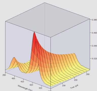
The spectrometer operating software can perform standard curve fitting of individual  $\Delta\text{OD}(t)$  curves. The standard analysis is based on exponential decay models, taking into account the Gaussian statistics of the raw data.
