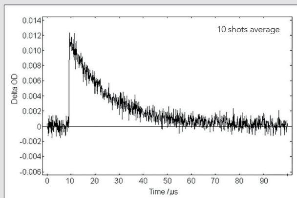
Demonstration of the detection limit and of the Signal-to-Noise improvement by signal averaging using the fast detector version
