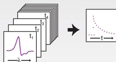
Spectrally resolved absorption kinetics can be extracted from spectral mode measurements by automatically stepping the gate delay through a predefined time range. Subsequent data slicing reveals the details of the transient absorption kinetics.
