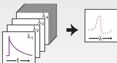
Time-resolved absorption spectra can be generated in kinetic mode laser flash experiments by automatic scanning through a pre-defined spectral range and subsequent data slicing. This technique requires many laser shots, in particular when high spectral resolution is required.
