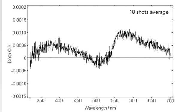
Demonstration of the detection limit and of the Signal-to-Noise improvement by signal averaging
