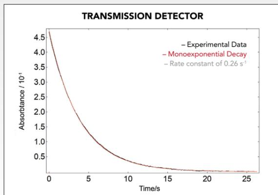
Bleaching of K<sub>3</sub>[Fe(CN)<sub>6</sub>] by Ascorbic Acid using the stopped-flow accessory. The absorption kinetic of Fe(CN)<sub>6</sub><sup>3-</sup> bleaching was recorded using the transmission detector of the FS5.
