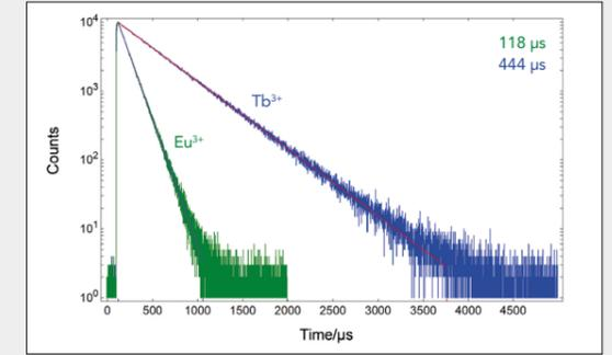
Luminescence decays of Tb<sup>3+</sup> and Eu<sup>3+</sup> ions and results of tail fit analysis. The samples were excited with the microsecond flashlamp.
