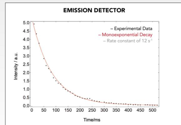
Fluorescence quenching of NATA by NBS using the stopped-flow accessory. The fluorescence kinetic of NATA quenching was recorded using the emission detector of the FS5.
