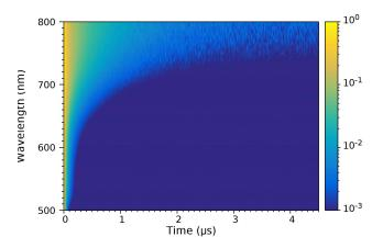
Figure 1 Time-resolved emission spectrum (TRES) of InP/ZnS QD solution measured using TCSPC. The photoluminescence intensity at each wavelength was normalised to 1. Experimental parameters:  $\lambda_{\text{ex}} = 405$  nm,  $\Delta\lambda_{\text{em}} = 15$  nm.
