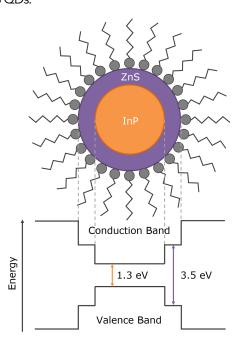
Figure 1 Structure and band energy diagram of core-shell InP/ZnS quantum
