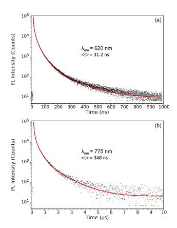
Figure 2 Photoluminescence decays measured at (a) 620 nm and (b) 775 nm. The decays were measured using TCSPC and fit with four exponentials components and the intensity weighted average lifetime calculated. Experimental parameters:  $\lambda_{ex} = 405$  nm,  $\lambda_{em} = 620$  nm / 775nm,  $\Delta\lambda_{em} = 10$  nm.
