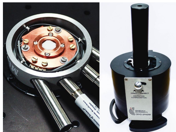
Figure 2: Sample holder (left) and integrating sphere (right) of the Cryosphere.
