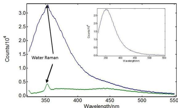
**Figure 1:** Subtraction of emission background and Raman scattering from raw fluorescence data. Spectrally corrected emission spectrum of porcine eye lens proteins in 7 M urea (50  $\mu$ m) (blue) and background (green) at 315 nm excitation wavelength. Protein emission spectrum after background subtraction (inset).
