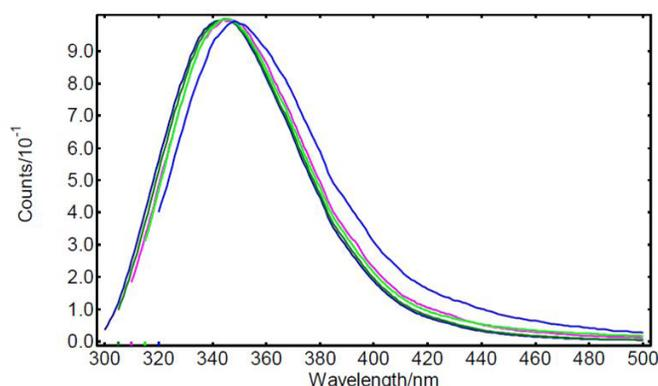
Figure 3: Emission spectra of NATA in glycerol at  $-10^{\circ}\text{C}$ . Excitation wavelength 295 nm, 300 nm, 305 nm, 310 nm and 315 nm.
