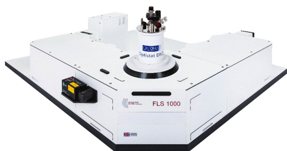
Figure 1 FLS1000 Photoluminescence Spectrometer equipped with an Oxford Instruments liquid nitrogen cryostat for the measurement of low-temperature phosphorescence spectra.
