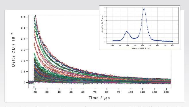
Raw data and fitted curves of the set of 80 time-resolved measurements of an anthracene example. Data were analysed with FLASH software (optional) using Global Analysis of a second order kinetic decay model, globally linking the rate constant. The result of the fit is a global second order rate constant of 1.8x10<sup>3</sup> (M ms)<sup>-1</sup> and a wavelength dependence of the amplitude as shown in the insert.
