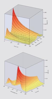
The spectrometer operating software can perform standard curve fitting of individual  $\Delta OD(t)$  curves. The standard analysis is based on exponential decay models, taking into account the Gaussian statistics of the raw data.
