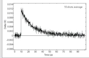
Demonstration of the detection limit and of the Signal-to-Noise improvement by signal averaging using the fast detector version
