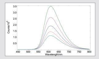
**Sample:** Ruthenium Bipyridine in water **Measurement Conditions:** (LIF)  $\lambda_{pump} = 450$  nm,  $E_{pump} = 10$  mJ, spectral range 450 nm - 800 nm, gate width = 100 ns
