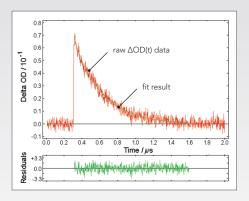
The sample being investigated is exposed to an intense laser pump pulse, which creates the transient species, and the probe source, which forms the background for the time dependent absorption measurement.
