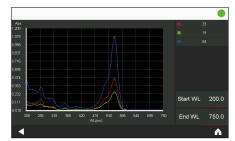
Measurement parameters, acquisition and analysis on DS5 touchscreen
