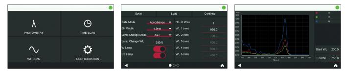
Measurement parameters, acquisition and analysis on DS5 touchscreen
