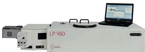
Figure 1: The Edinburgh Instruments LP980 Spectrometer.
