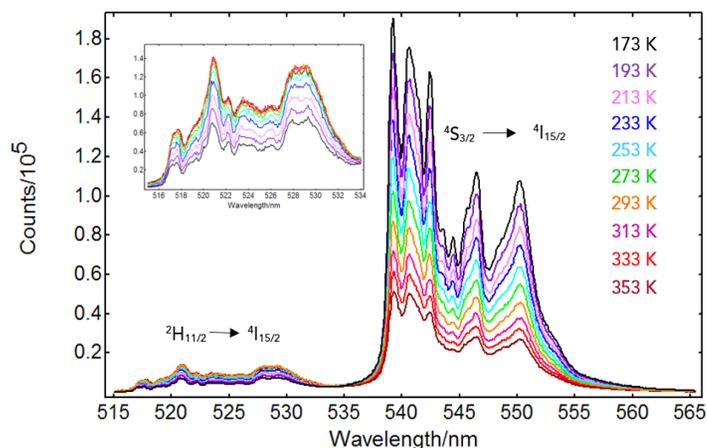
**Figure 2:** Temperature emission map of  $\text{NaY}_{0.77}\text{Yb}_{0.20}\text{Er}_{0.03}\text{F}_4$  measured with Linkam stage in FLS1000, green upconversion emission. Conditions:  $\lambda_{\text{ex}} = 980 \text{ nm}$ ,  $\Delta\lambda_{\text{ex}} = 10 \text{ nm}$ ,  $\Delta\lambda_{\text{em}} = 0.20 \text{ nm}$ , step size =  $0.10 \text{ nm}$ , integration time =  $1 \text{ s/step}$ . The inset shows the  $2\text{H}_{11/2} / 4\text{I}_{15/2}$  region in detail.
