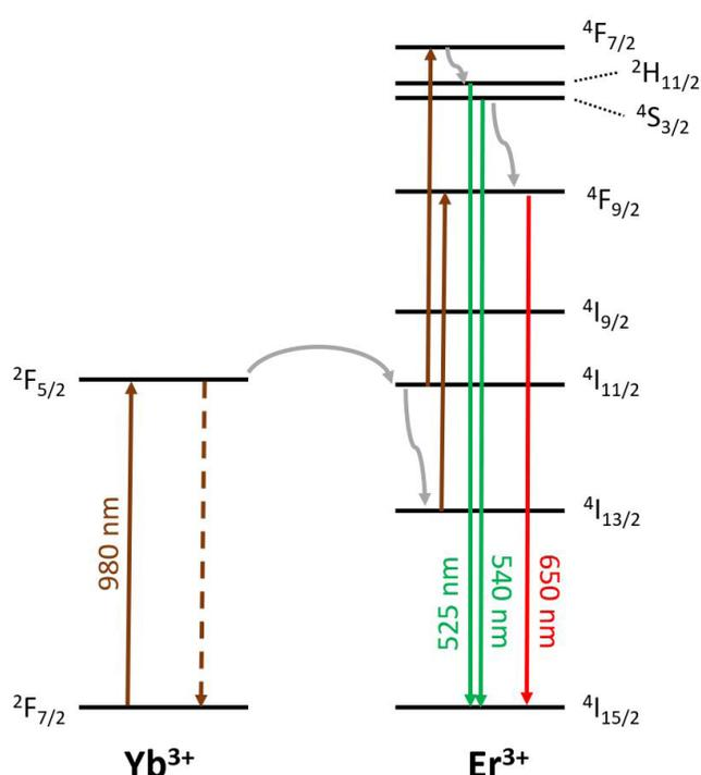
**Figure 1:** Schematic of upconversion mechanism in  $\text{NaY}_{0.77}\text{Yb}_{0.20}\text{Er}_{0.03}\text{F}_4$ , showing green and red luminescence transitions. Grey arrows indicate nonradiative processes.
