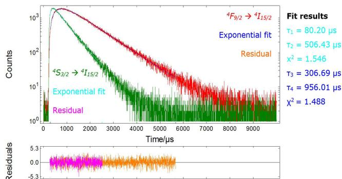
**Figure 4:** Decay on curves of the  ${}^4\text{S}_{3/2}$  and  ${}^4\text{F}_{9/2}$  to  ${}^4\text{I}_{15/2}$  (green and red, respectively) upon 976.4 nm and 30  $\mu\text{s}$  pulsed excitation.
