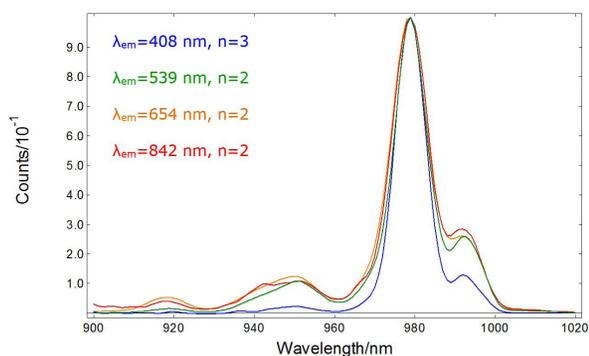
**Figure 3:** Excitation spectra from 900 nm to 1020 nm at the peak wavelengths of the main emission bands. The experimental conditions were  $\Delta\lambda_{\text{exc}} = 15$  nm,  $\Delta\lambda_{\text{em}} = 5$  nm and a step of 1 nm.
