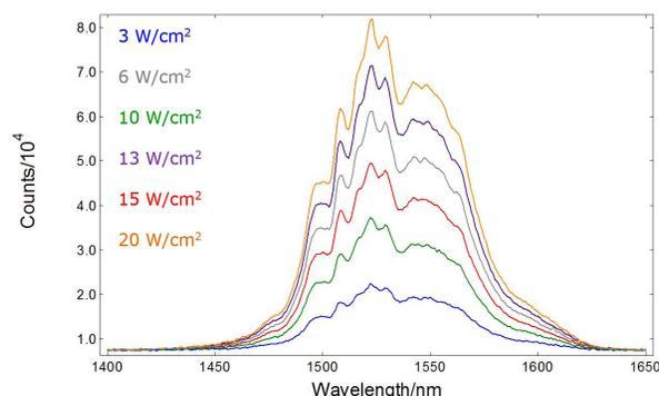
**Figure 2:** Emission spectra of  $\text{NaYF}_4:\text{Yb}^{3+}\text{Er}^{3+}$  from the  $^4I_{13/2} - ^4I_{15/2}$  upon 976.4 nm excitation.  $\Delta\lambda_{em}=0.5$  nm, step=1 nm
