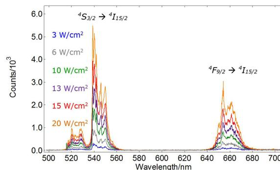
**Figure 1:** Emission spectra of  $\text{NaYF}_4:\text{Yb}^{3+}\text{Er}^{3+}$  from  $^4S_{3/2}$  and  $^4F_{9/2}$  to  $^4I_{15/2}$  upon 976.4 nm excitation.  $\Delta\lambda_{em}=0.1$  nm, step=0.2 nm
