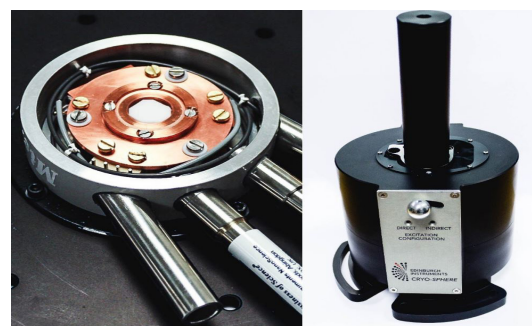
Figure 2: Variable temperature sample holder (left) and side view of Edinburgh Instruments Cryosphere accessory (right).
