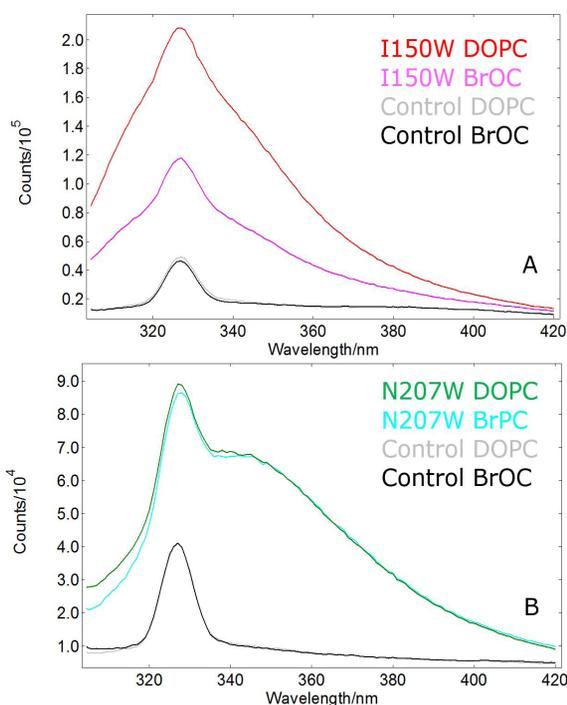
**Figure 1:** Emission spectra of brominated and non-brominated lipids with lipid-only controls. The samples were excited at 295 nm with  $\Delta\lambda_{exc} = 3$  nm and  $\Delta\lambda_{em} = 7$  nm,  $Pol_{exc} = 90^\circ$ ,  $Pol_{em} = 0^\circ$ , step = 1 nm,  $t_{integr} = 1$  s.
