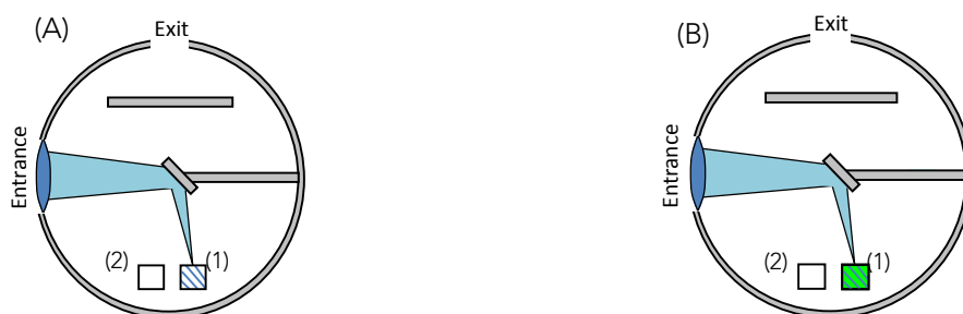
Figure 10. Two different measurement configurations required for Direct Excitation measurements: (A) reference sample (solvent only) in sample position (1); (B) test sample in position 1 (position 2 remains empty for both measurements.)
