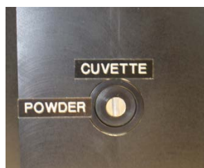
Figure 5. Two position mirror dial set for liquid samples measurements
