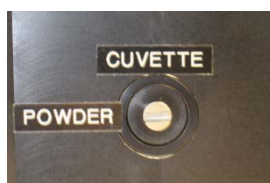
Figure 8. Two position mirror dial set for solid samples measurements
