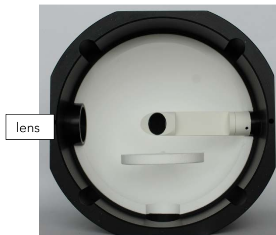
Figure 9. View into the upper half of the sphere; setup for solid samples measurements
