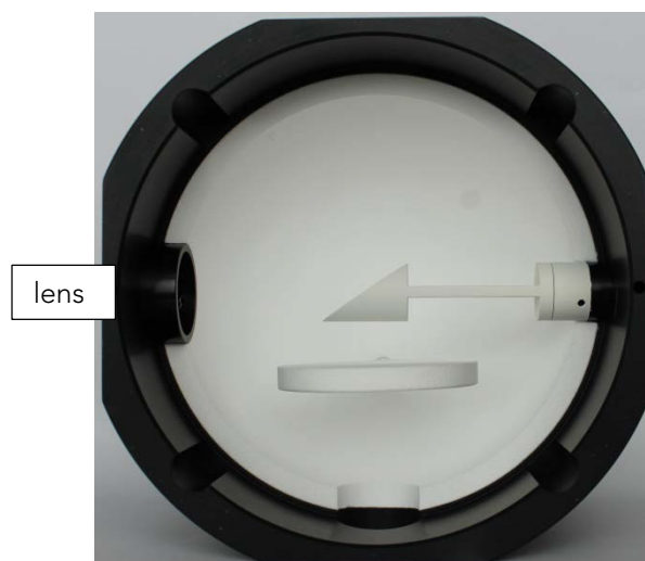
Figure 6. View into the upper half of the sphere half; setup for liquid samples measurements
