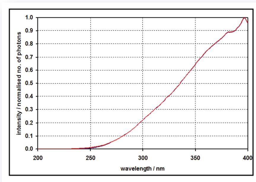
Fig. 2 Normalised excitation correction curves for a lamp fitted with an ozone free bulb (blue) and ozone generating bulb (red); the excitation monochromator is fitted with a 1200g/mm, ruled, 300nm blazed grating
