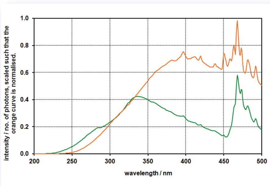
Fig. 1. Excitation correction curves for two different grating sets in a double excitation monochromator.
