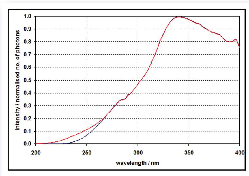
Fig. 3 Normalised excitation correction curves for a lamp fitted with an ozone free bulb (blue) and ozone generating bulb (red); the excitation monochromator is fitted with a 1800g/mm, holographic, 250nm optimised grating
