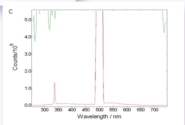
Figs. 1a, 1b & 1c. Comparison of measurements of scatter taken with an FLS980 with single monochromators and (green curve), an FLS980 with double monochromators (red curve) and the peak measurement taken with an ND filter (blue curve). Shown scaled differently over three graphs to allow the peak to be seen and the background to be shown on measurements from both spectrometers.
