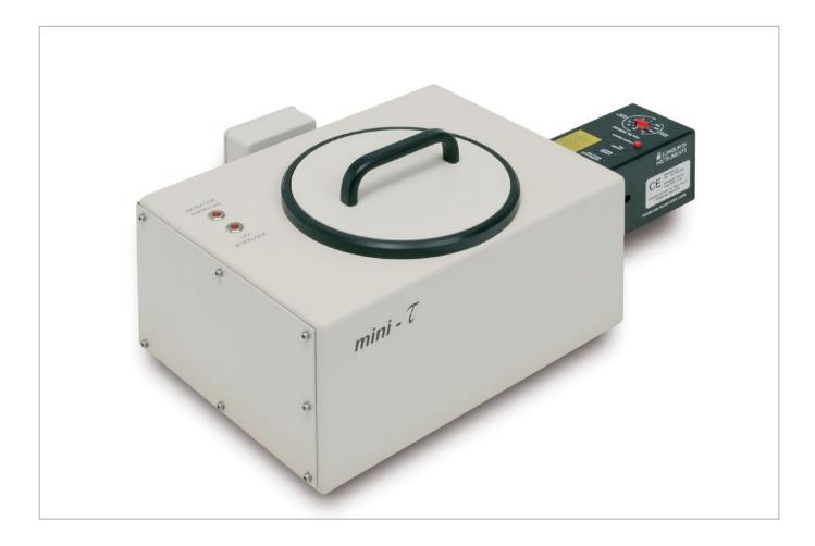
The mini-t is an ultra-compact, low cost, filter based fluorescence lifetime spectrometer. Using the Time Correlated Single Photon Counting (TCSPC) technique, the Mini-tau is supplied with F980 software and a TCC2 electronics module to enable fast, reliable and accurate measurement and data analysis.
