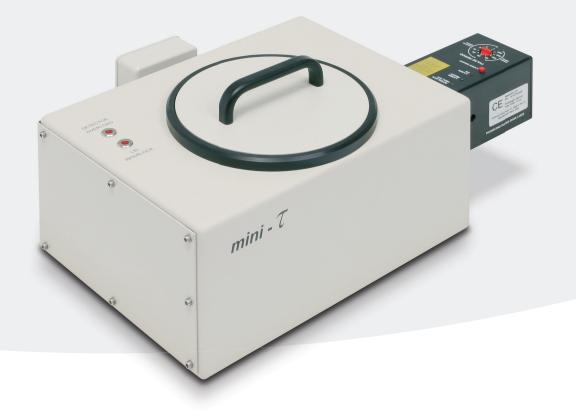
The Mini-tau is an ultra-compact, low cost, filter-based dedicated fluorescence lifetime spectrometer. Using the Time-Correlated Single Photon Counting (TCSPC) technique, the Mini-tau can measure fluorescence lifetimes ranging from 25 ps to 10 µs.
