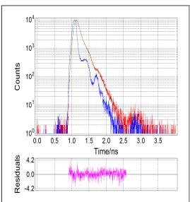
Erythrosin B in water, excitation by supercontinuum laser at 520nm, detection by MCP-PMT at 560nm. The calculated lifetime is (88±2) ps, with a goodness of fit quality parameter ( $\chi^2$ ) of 1.180.
