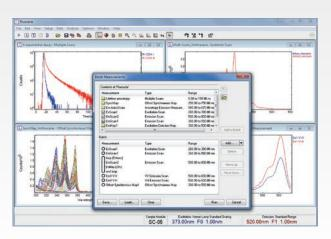
Analysis methods such as photoluminescence quantum yield, chromaticity coordinates, absorption, or anisotropy are implemented in user-friendly wizards. Analysis of time-resolved photoluminescence is straightforward in Fluoracle: up to 4 exponential components can be fitted to fluorescence or phosphorescence decays instantly. Reconvolution fitting, shift and offset fitting, and fit quality parameters are provided as standard.
