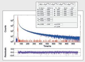
TCSPC decay and fit result in Fluoracle
