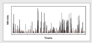
Typical pulses from a single photon counting photomultiplier. Only photon pulses above a certain threshold value are counted. This eliminates unstable background and associated noise.
