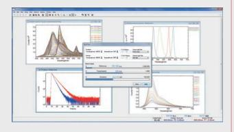
Batch acquisition is available in Fluoracle. The user can program a sequence of measurements including delays, loops, temperature or sample changes (accessory dependent). Batch files can be saved and loaded when needed.
