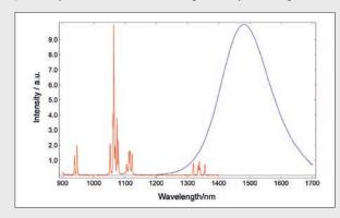
Peak-normalised spectra acquired with two different detector options in the NIR range: emission from PbS quantum dots in toluene with NIR+ (blue), and from Nd:YAG with NIRA+ (red). The analogue detector option (NIRA+) is suitable for high fluorescence intensities, while samples with low quantum yield benefit from a photon-counting detector (NIR+).
