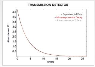
Bleaching of  $K_a[Fe(CN)_{\lambda}]$  by Ascorbic Acid using the stopped-flow accessory. The absorption kinetic of  $Fe(CN)_{\lambda}^{3}$  bleaching was recorded using the transmission detector of the FS5.
