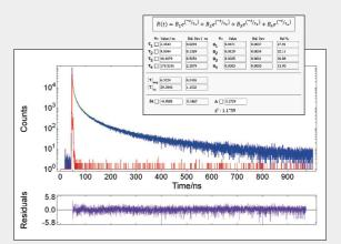
TCSPC decay and fit result in Fluoracle.
