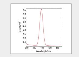
Sensitivity is generally specified by the Raman spectrum of water, excited at 350 nm, spectral bandwidths of 5 nm in excitation and emission, integration time of 1 s.
