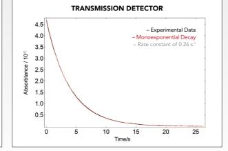
Bleaching of  $K_4$ [Fe(CN)<sub>6</sub>] by Ascorbic Acid using the stopped-flow accessory. The absorption kinetic of Fe(CN)<sub>6</sub><sup>3-</sup> bleaching was recorded using the transmission detector of the FS5.
