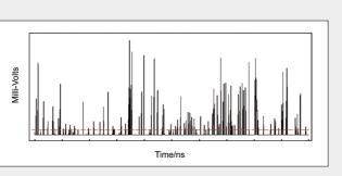
Typical pulses from a single photon counting photomultiplier. Only photon pulses above a certain threshold value are counted. This eliminates unstable background and associated noise.
