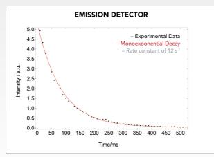
Fluorescence quenching of NATA by NBS using the stopped-flow accessory. The fluorescence kinetic of NATA quenching was recorded using the emission detector of the ES5.
