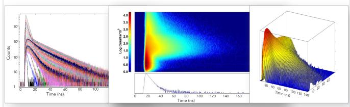
Sample: Norharman in methanol (5×10<sup>-5</sup>M) Excitation Source: 280 nm pulsed LED (EPLED-280)
