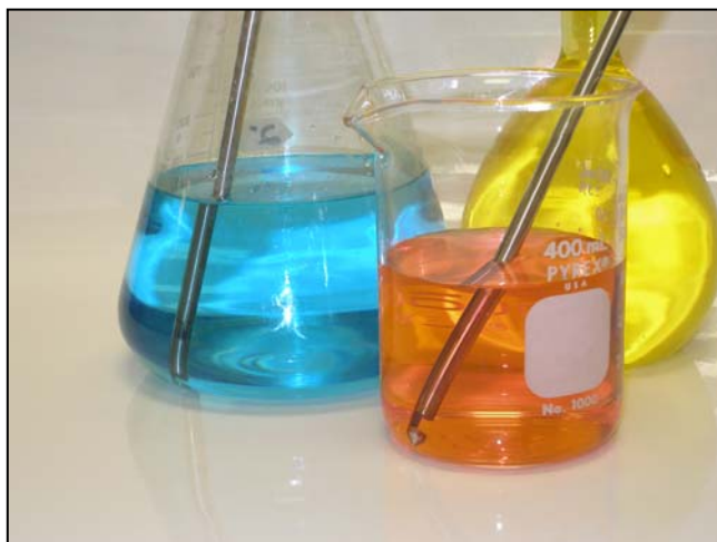
Dip probes used to measure color, concentration, or kinetics of liquids
