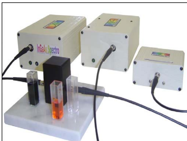
UV-VIS-NIR system covering 280-1700nm range, with cuvette accessory
